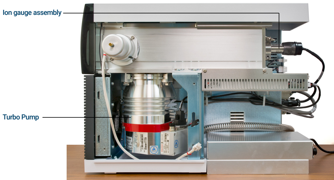
Figure 58. Turbo pump and related parts
