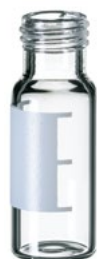
11 40 2556 HPLC/GC Certified Vial Kit: 1.5ml Short Thread Vial, 32 x 11.6mm, clear glass, 1 st hydrol. class, label; UltraClean Closure: 9mm PP Short Thread Cap, blue, centre hole; Silicone white/PTFE red, 55° shore A, 1.0mm
