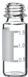
11 40 3196 LC/MS and GC/MS Certified Vial Kit: 1.5ml Short Thread SureStop™ Vial, 32 x 11.6mm, clear glass, wide opening, with overwind-barrier; Ultra High Performance Seal: PP Short Thread Cap, blue, centre hole; Silicone darkblue-translucent/PTFE natural, 35° shore A, 1.0mm
